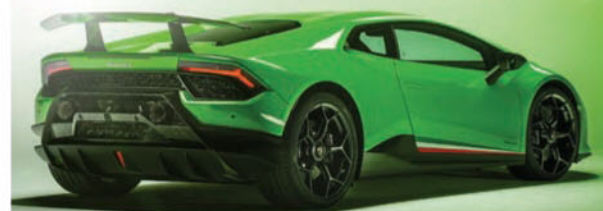
Active rear wing can direct air left or right to optimise cornering
