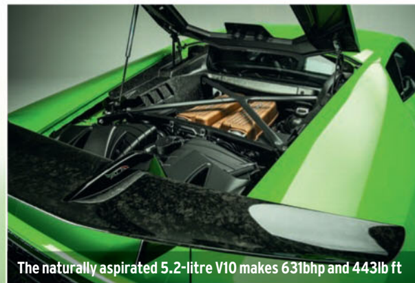
Active rear wing can direct air left or right to optimise cornering
